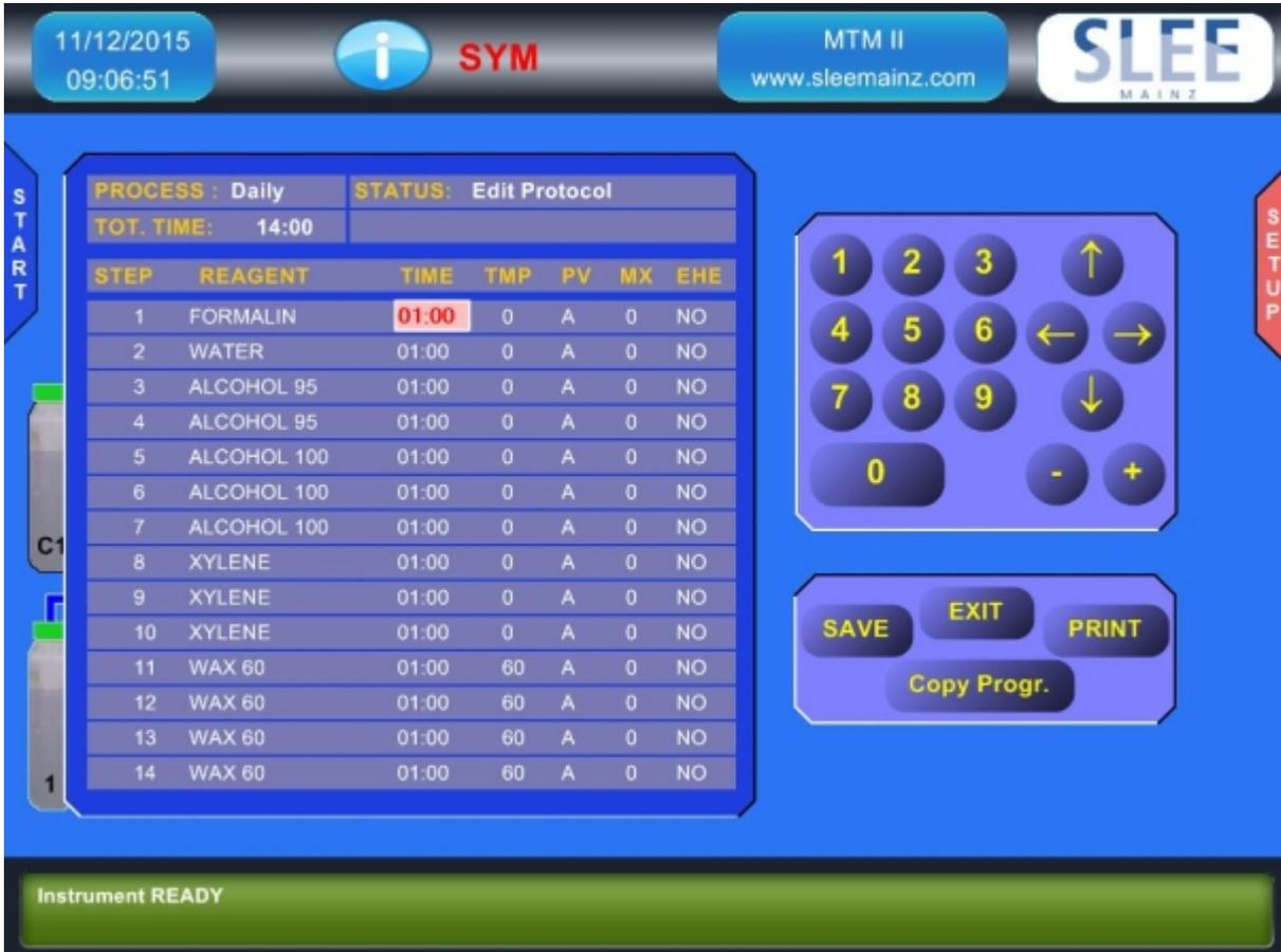
With the ARROW keys it will be possible to “navigate” the entire program to select the field to edit. Each field content can be varied by using the extended character keyboard or, in some cases, by using the +/- keys.
