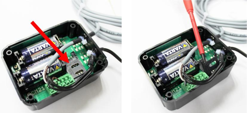
Two close-up images of the SIM card holder. The left image shows a red arrow pointing to the holder. The right image shows a red screwdriver being used to pry open the lid of the holder.                                                          |
