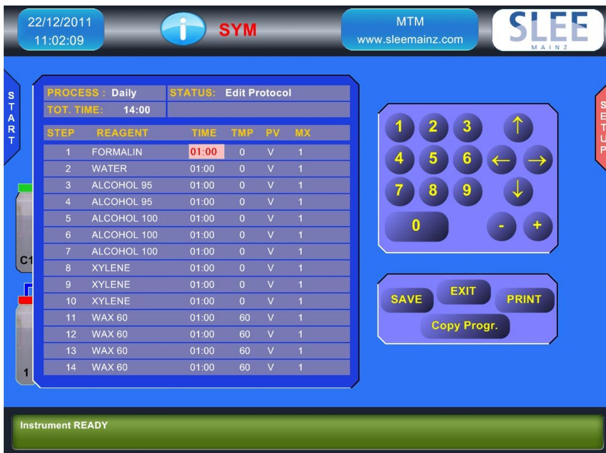
With the ARROW keys it will be possible to "navigate" through the entire program to select the field to edit. Each field content can be varied by using the extended character keyboard or, in some cases, by using the + / - keys.
