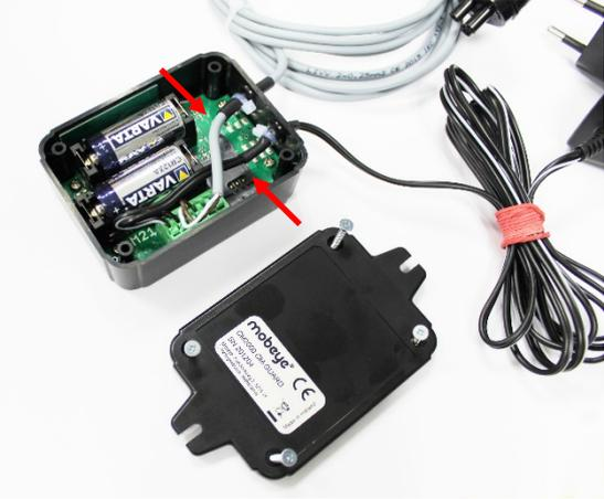
The device is shown with its lid removed. The internal green PCB is visible, featuring two VARTA batteries and a SIM card holder. Red arrows point to the SIM card holder and the internal components. The lid is placed to the right of the device. |
