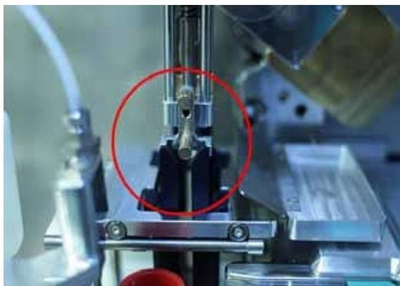
This picture again shows the adjustment-wheel for the coverglass position. When the position is perfectly adjusted, you will need to check if the separation pressure (bending the coverglass) (fig. 1) is optimized to your coverglass, as every glass has different flexibility and separation characteristics! This is explained in the next step.
