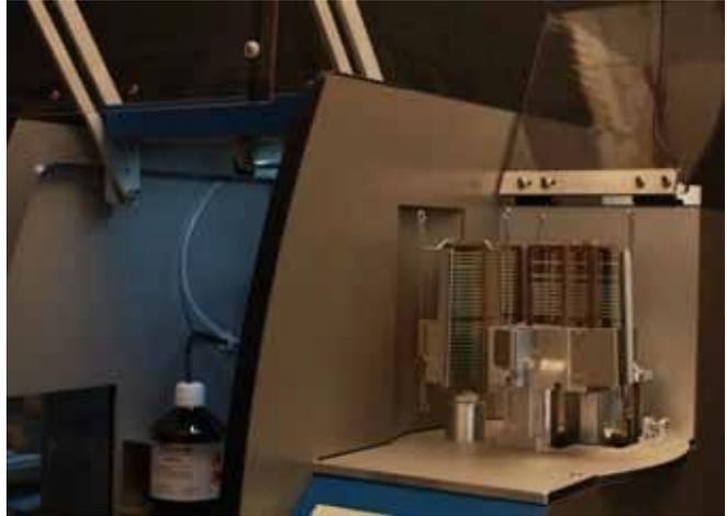
The MCS I checks for free storage positions regularly. So if it detects 4 full stations, it will inform the user with a message in the display and a small alarm, to be sure somebody will empty the positions.
