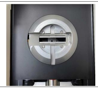
Now you can see the x / y orientation system. For inserting the excenter ring, the x position must be in a 0-axis position and the y position must be in a 0 position as well.
