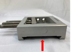
All of the basic object holders have guidelines for dovetails. Like this you can use the full width of your knives with all applications.
