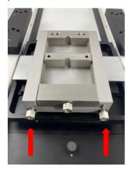
To fix the object plate at any place on the lateral movement, tighten both Allen key screws.
