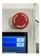
By pressing the emergency stop button you immediately freeze all moving parts of the device. Hit the button to activate the emergency stop to prevent any dangerous situation.
