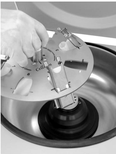
Removal of Cellcliprotor out of the centrifuge.
