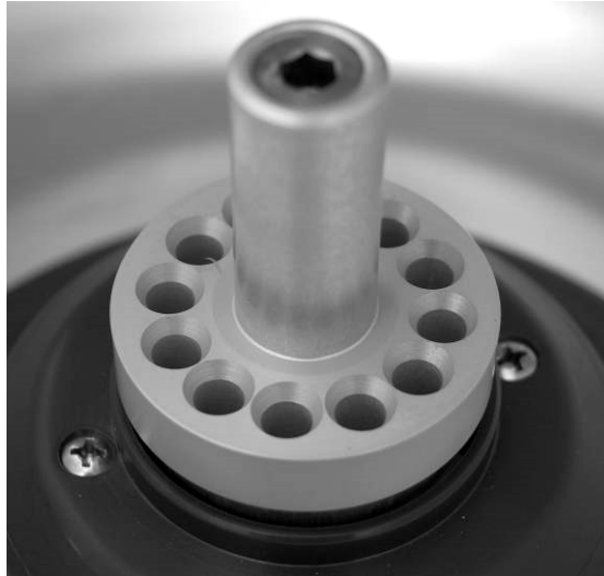
Safety pin lock at the centrifuge hub.
