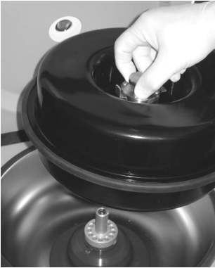
Removal of closed rotor out of the centrifuge.
