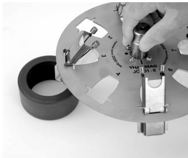
Placement of Cellcliprotor onto the rotor holder.
