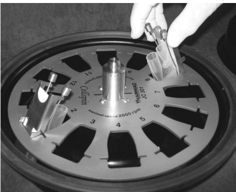
Loading of closed rotor.
