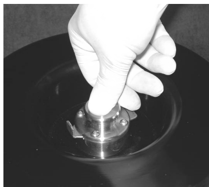
Closing of rotor lid.
