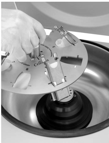
Removal of Cellcliprotor out of the centrifuge.
