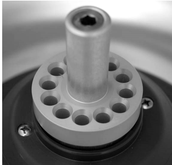
Safety pin lock at the centrifuge hub.
