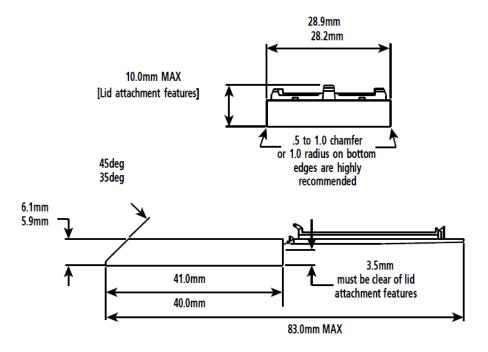
Cassettes may have lids attached in the open position as shown, lids may be removed or lids may be in a closed position as long as they do not project over
