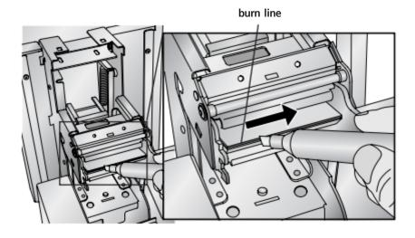
To prevent damage to print head, do not touch the burn line with a finger ring containing diamond or metal.
