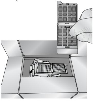
3. Depending on the mode that is set in the PTLab software, the printer will print on the cassette as soon as it detects its presence or wait for the user to press the cassette (bottom) button next to the flashing LED light (default setting).
