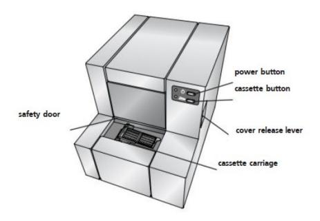
The **cover release lever** is a mechanical lever that releases the spring-loaded mechanism on the cover. Pull it toward the front of the printer to release the cover latch.
